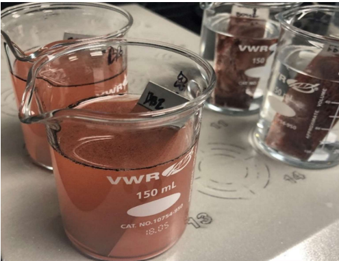
Photo 1: degreasing test of one surfactant in process, in foreground, and another surfactant starting in background
