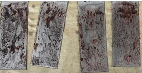
Photo 2: degreasing test completed for two surfactants and their respective coupons after simulated rinsing
